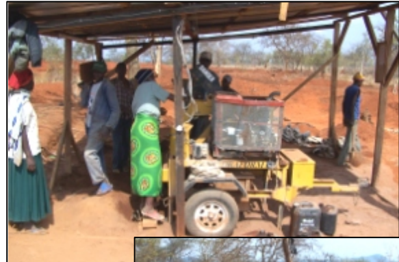
The hydraform and its capabilities to make blocks using locally obtained materials eg, loam soil, water & cement
